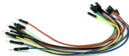
Figure 12: Jumper wires
