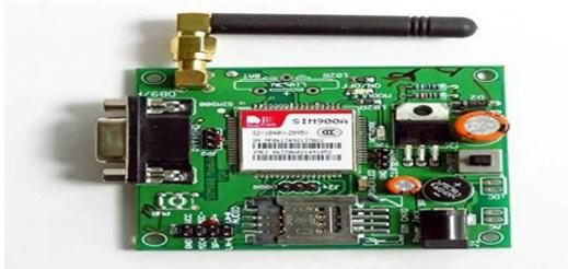
Figure 10: GSM module
